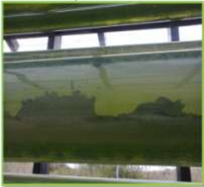
Biofilm in PBR Before use of Spiked Balls
